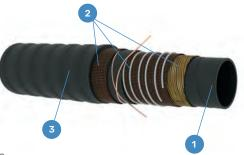
The above drawing illustrates a hose designed to resist pressure. For applications requiring resistance to vacuum, and suction, a steel wire helix is embedded into the hose body. The spiral also increases the flexibility of the hose.
