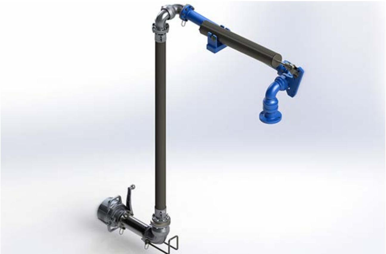
Because of the robust and high quality design of the swivel joints and the precise loading arm balancing, handling of the loading arm is very easy. Recent developments have allowed for six swivels to be used in each arm. This gives true three axis movement at the tanker connection and makes handling the arm valves or accessories effortless.
