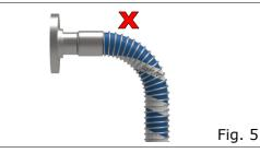
**BENDING RADIUS:** Installation tighter than the minimum bending radius reduces the life of the hose considerably. Moreover it is necessary to avoid bending close to the end fittings. (Fig. 5 & 6)
