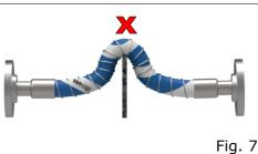
**INSTALLATION:** The hoses must be supported to allow normal movement when under pressure (dimensional variations).
